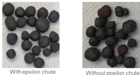
Figure 12: Impact of the use of TDRF on pellets sphericity (Results are courtesy of ArcelorMittal Mines Canada – Pellet Plant)
