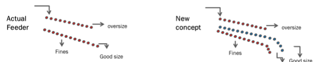
Figure 4: Concept of using an intermediate deck to increase screening area for the same physical space of the double deck
