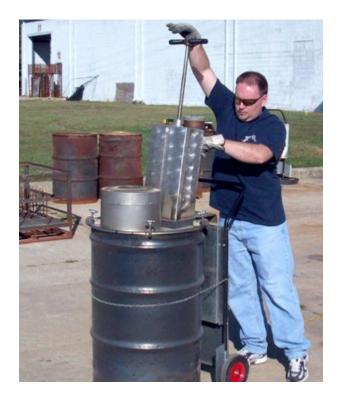
The Easy Feed Cartridge allows operators to inject refuse into the barrel while the unit is in operation.
